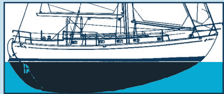
4. Full Keel low drift rate, high drag.
